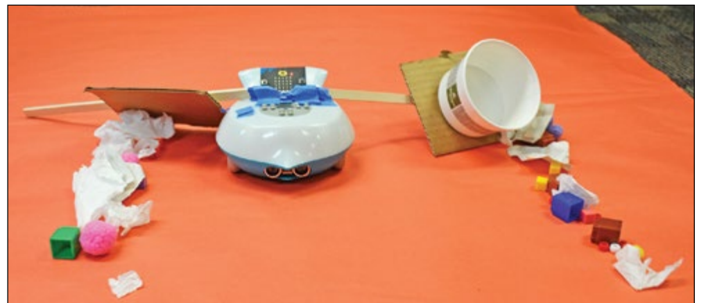
This Finch Robot uses long arms to sweep up trash. It is a project of Daniel Marquez, Joselyn Navarro, Richard Hernandez and Brisa Reynolds.
