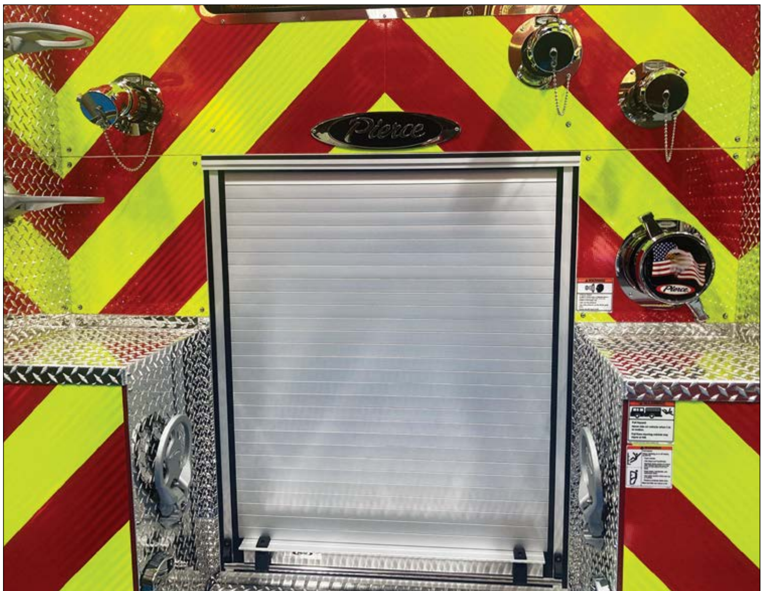
The intakes on the back of the new fire engine are shown in this photo.
