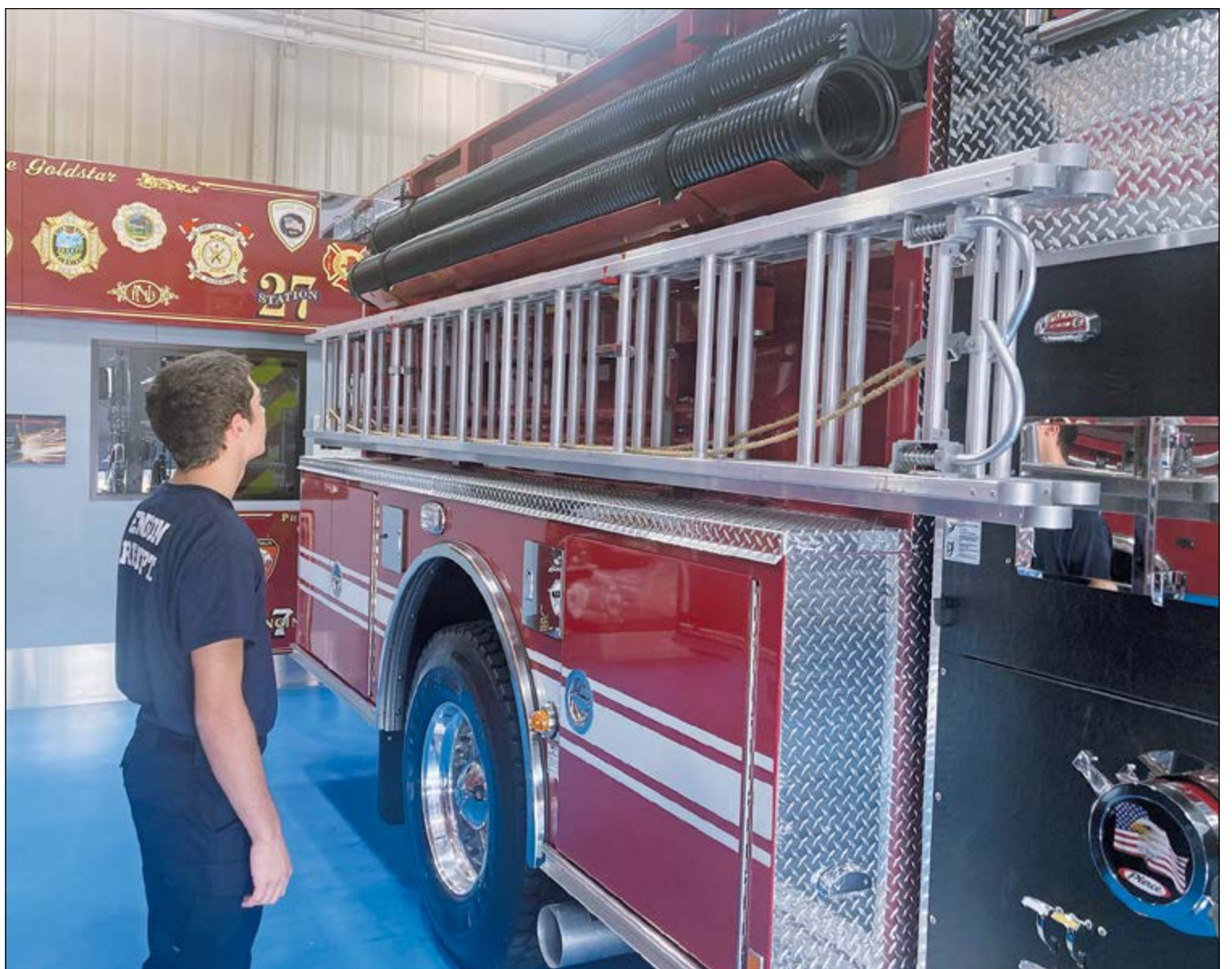
Eli Snowgren, son of Denison Fire Chief Cory Snowgren, looks at the ladders and hard suction lines that are mounted on the right side of Denison's new fire engine. On the old engine, that equipment was mounted on the top, making it more difficult to put into service.
